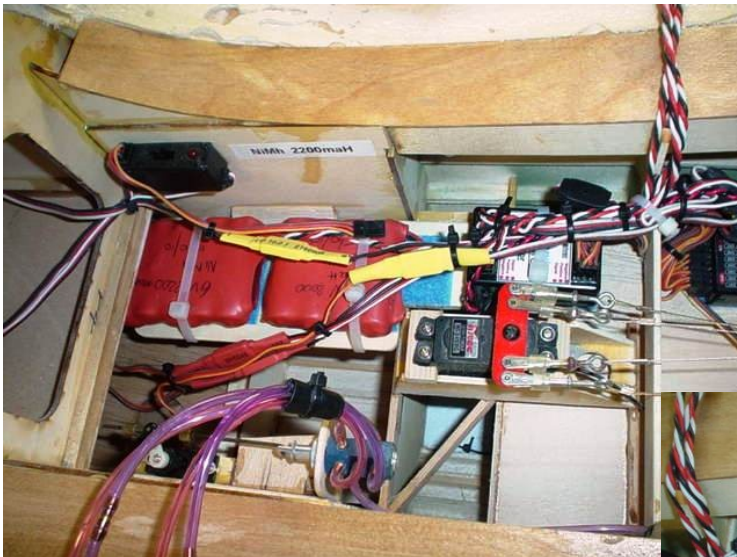
Batteries are made up from low self discharge NiMH cells of 2200mah capacity. One battery of 4.8V powers the receiver exclusively and the other of 6V powers the servos exclusively. A further identical 4.8V pack mounted forward of the firewall powers the ignition.
